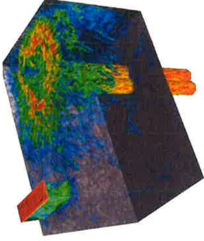
This image simulates flow into an advanced recycling nuclear reactor.
